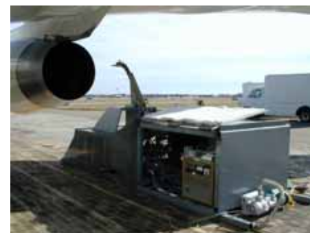
Sampling platform for jet engine exhaust aerosol characterization experiment
