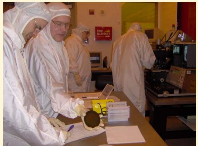
Steve Anderson and Kevin Cleare record wafer preparation information, while Kathy Hough observes Bill Fish (seated behind instructor Kevin Roberts), aligning a wafer and mask with the MA/BA-6 aligner.
