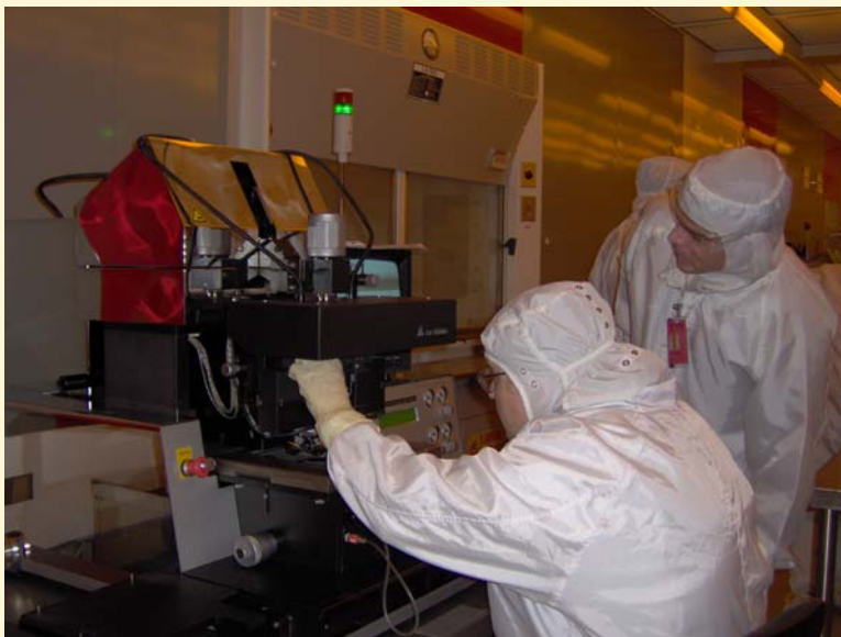
Kathy Hough with instructor Kevin Roberts aligning a wafer to a mask on the MA/BA-6 aligner. This was part of week ten's Final Project during which students made cantilever beams in silicon nitride.
