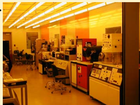
Bay 3 of NFC, some of the plasma processing tools in the cleanroom
